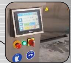
The control panel with a multi language touch screen.
