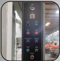
Automatic timer controls. Optional PLC/HMI touchscreen available.
