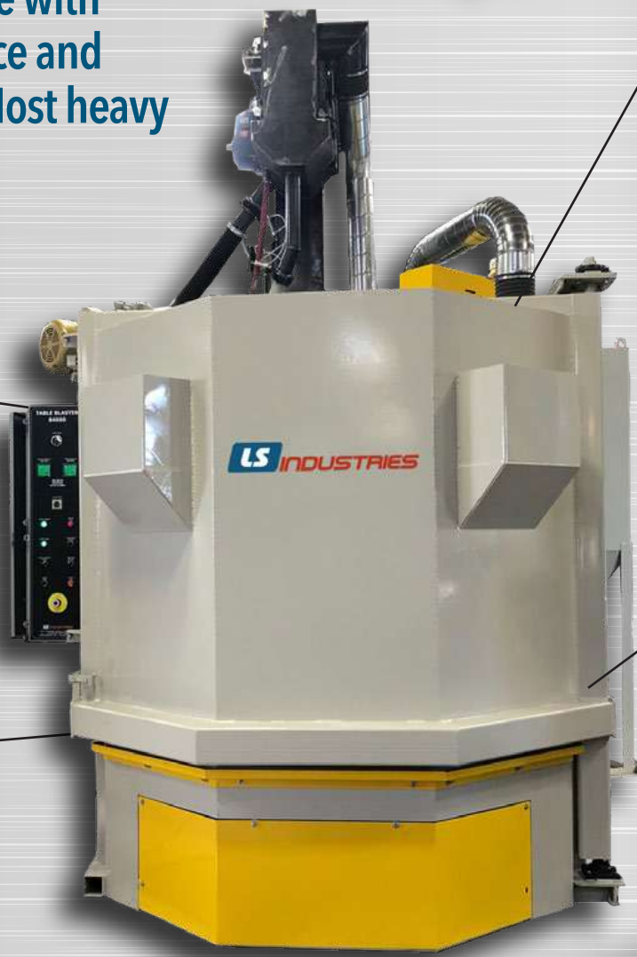
Hinge mounted doors with manganese replaceable, wear resistant liners.
