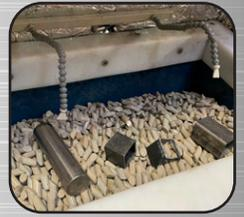
Comes with adjustable hoses to spray solution on the media to help clean the parts.
