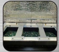
Optional dividers for separated parts finishing. UHMW Tub liners eliminates scratching of parts
