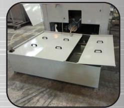
We offer an optional tank for easy removal of dirt solution.
