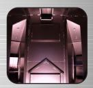
The blaster is designed for long life as well with the heavy-duty manganese blast cabinet and easily replaceable manganese wear liners.
