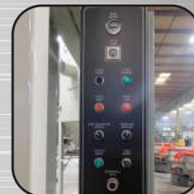
Automatic timer controls. Optional PLC/HMI touchscreen available.
