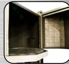
Hinge mounted doors with manganese replaceable, wear resistant liners.
