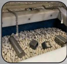
Comes with adjustable hoses to spray solution on the media to help clean the parts.
