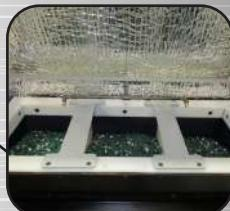
Optional dividers for separated parts finishing. UHMW Tub liners eliminate scratching of parts.
