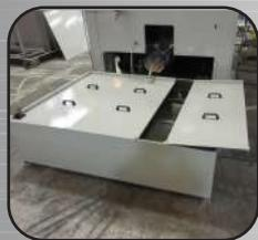
We offer an optional tank for easy removal of dirt solution.
